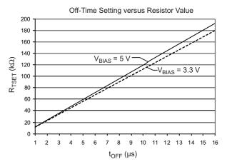
The  $R_{TSET}$  resistor should be not smaller than 7.65 k $\Omega$  ±2% to prevent very short off-times from violating the minimum on-time of the switcher.
