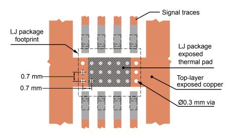
Suggested PCB layout for thermal optimization (maximum available bottom-layer copper recommended)
