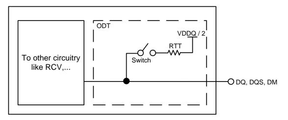
The switch is enabled by the internal ODT control logic, which uses the external ODT pin and other control information. The value of RTT is determined by the settings of Mode Register bits. The ODT pin will be ignored if the Mode Register MR1 and MR2 are programmed to disable ODT and in self-refresh mode.
