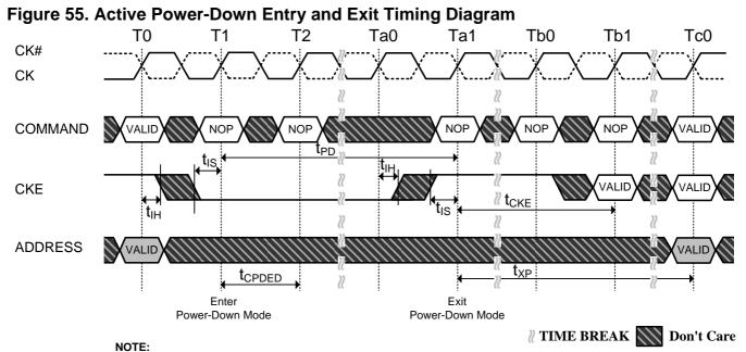
VALID command at T0 is ACT, NOP, DES or PRE with still one bank remaining open after completion of the precharge command.
