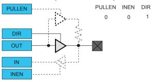
Figure 23-7. I/O Configuration - Totem-Pole Output with Enabled Input
