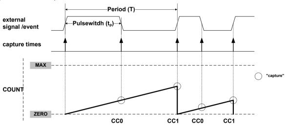
Selecting PWP or PPW in the Timer/Counter Event Input 1 Action bit group in the Event Control register (EVCTRL.EVACT1) enables the TCC to perform one capture action on the rising edge and the other one on the falling edge. When using PPW (period and pulse-width) event action, period T will be captured into CC0 and the pulse-width  $t_p$  into CC1. The PWP (Pulse-width and Period) event action offers the same functionality, but T will be captured into CC1 and  $t_p$  into CC0.
