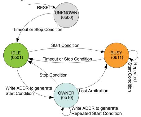
The bus state machine is active when the I<sup>2</sup>C master is enabled.
