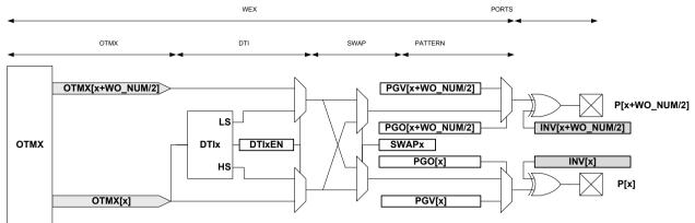
**The output matrix (OTMX)** unit distributes compare channels, according to the selectable configurations in Table 31-4.
