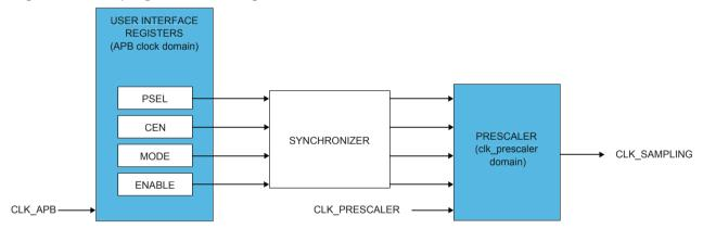
The BOD33 Clock Enable bit (BOD33.CEN) in the BOD33 register and the BOD12 Clock Enable bit (BOD12.CEN) in the BOD12 register should always be disabled before changing the prescaler value. To change the prescaler value for the BOD33 or BOD12 during sampling mode, the following steps need to be taken:
