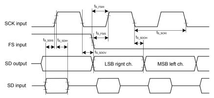
Figure 44-7. I2S Timing PDM2 Mode
