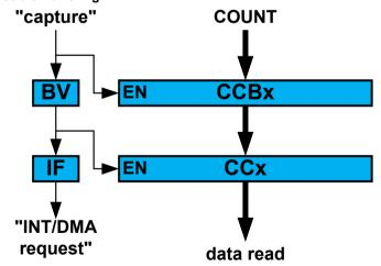
The TCC can detect capture overflow of the input capture channels: When a new capture event is detected while the Capture Buffer Valid flag (STATUS.CCBV) is still set, the new timestamp will not be stored and INTFLAG.ERR will be set.
