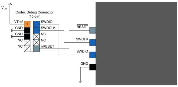
Table 39-10. Cortex Debug Connector (10-pin)
