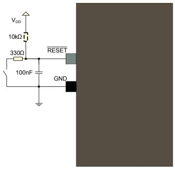
A pull-up resistor makes sure that the reset does not go low unintended causing a device reset. An additional resistor has been added in series with the switch to safely discharge the filtering capacitor, i.e. preventing a current surge when shorting the filtering capacitor which again causes a noise spike that can have a negative effect on the system.
