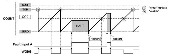
Figure 31-29. Waveform Generation with Fault Qualification, Halt, and Restart Actions
