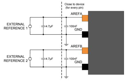
Figure 39-3. External Analog Reference Schematic With One Reference
