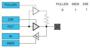
Figure 23-8. I/O Configuration - Output with Pull
