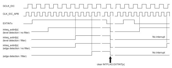
The detection delay depends on the detection mode.
