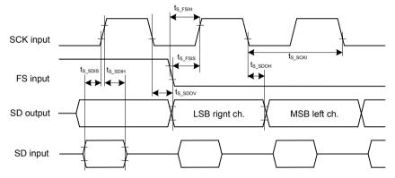
Figure 37-26. I2S Timing PDM2 Mode
