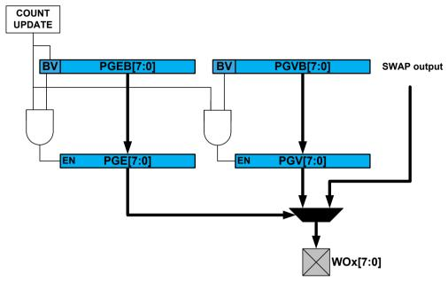
As with other double-buffered timer/counter registers, the register update is synchronized to the UPDATE condition set by the timer/counter waveform generation operation. If synchronization is not required by the application, the software can simply access directly the PATT.PGE, PATT.PGV bits registers.
