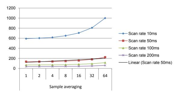
Figure 37-10. Power Consumption [μA] 10 sensors, noise countermeasures Enabled, f=48MHz, Vcc=3.3V
