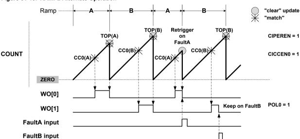
Figure 31-19. RAMP2 Alternate Operation
