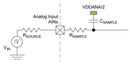
To achieve n bits of accuracy, the  $\mathcal{C}_{\mathrm{SAMPLE}}$  capacitor must be charged at least to a voltage of
