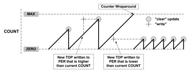
Figure 30-8. Changing the Top Value with Down-Counting Operation
