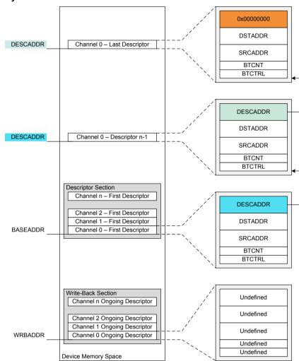
The size of the descriptor and write-back memory sections is dependent on the number of the most significant enabled DMA channel m, as shown below:
