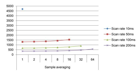
Figure 37-12. Power Consumption [μA] 100 sensors, noise countermeasures Enabled, f=48MHz, Vcc=3.3V
