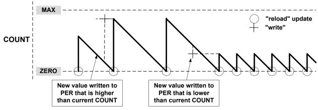
A counter wraparound can occur in any operation mode when up-counting without buffering, see Figure 31-10. COUNT and TOP are continuously compared, so when a new value that is lower than the current COUNT is written to TOP, COUNT will wrap before a compare match.
