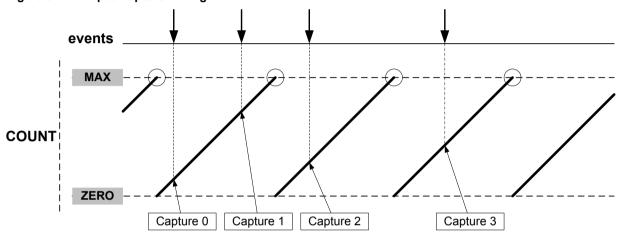
For input capture, the buffer register and the corresponding CCx act like a FIFO. When CCx is empty or read, any content in CCBx is transferred to CCx. The buffer valid flag is passed to set the CCx interrupt flag (IF) and generate the optional interrupt, event or DMA request. CCBx register value can't be read, all captured data must be read from CCx register.
