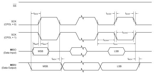
Figure 37-21. SPI Timing Requirements in Slave Mode
