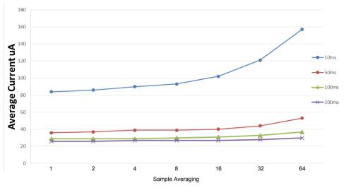
Figure 37-16. 10 Sensor / PTC\_GCLK = 4MHz / FREQ\_MODE\_NONE
