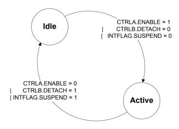
In Idle state, the pad is in low power consumption mode.
