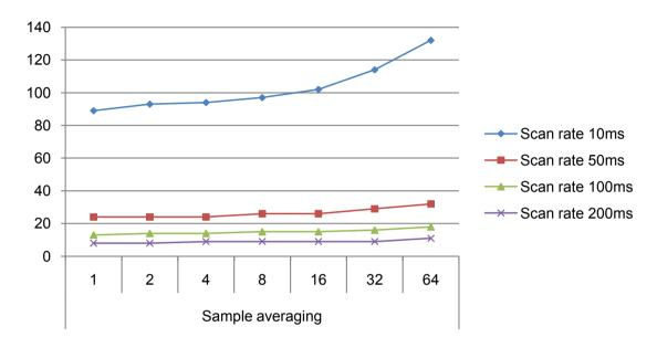
Figure 37-8. Power Consumption [μA] 1 sensor, noise countermeasures Enabled, f=48MHz, Vcc=3.3V
