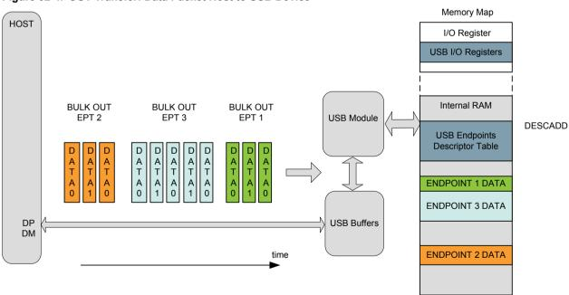
When an OUT token is detected, and the device address of the token packet does not match DADD.DADD, the packet is discarded and the USB module returns to idle and waits for the next token packet.
