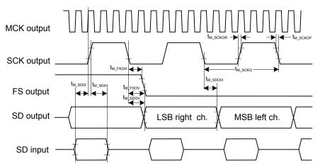
Figure 37-25. I2S Timing Slave Mode
