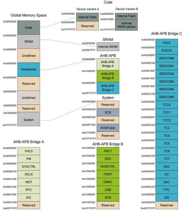
This figure represents the full configuration of the Atmel<sup>®</sup> SAM D21 with maximum flash and SRAM capabilities and a full set of peripherals. Refer to the Configuration Summary for details.
