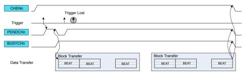
If the trigger source generates a transfer request for a channel during an ongoing transfer, the new transfer request will be kept pending (CHSTATUS.PEND=1), and the new transfer can start after the ongoing one is done. Only one pending transfer can be kept per channel. If the trigger source generates more transfer requests while one is already pending, the additional ones will be lost. All channels pending status flags are also available in the Pending Channels register (PENDCH).
