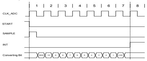
The sampling time can be increased by using the Sampling Time Length bit group in the Sampling Time Control register (SAMPCTRL.SAMPLEN). As example, the next figure is showing the timing conversion.
