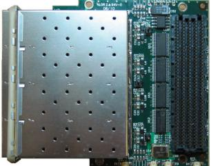
The FM-S18 is electrically compliant with the FMC standard. Due to the size of the quad SFP cages, the FM-S18 is classified as a mechanical superset of the FMC mechanical standards. Special attention should be paid to ensure that the FM-S18 is mechanically compatible if used with non-supported host carrier cards.
