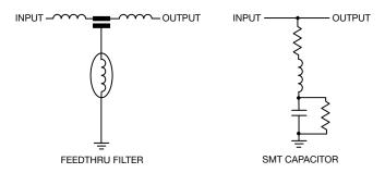
Figure 2. Comparison of Feedthru Capacitors to Discrete Capacitors
