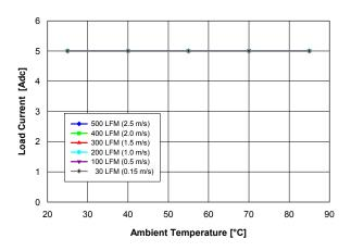
Fig. 0.7525V.2: Available load current vs. ambient temperature and airflow rates for Vout = 0.7525 V converter mounted horizontally with Vin = 5 V, air flowing from pin 5 to pin 1, and maximum MOSFET temperature  $\leq$  120 °C.
