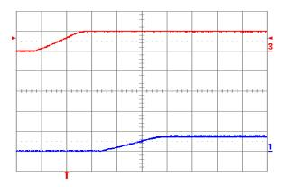
Fig. 0.7525V.4: Turn-on transient for Vout = 0.7525 V with application of Vin at full rated load current (resistive) and 47  $\mu$ F external capacitance at Vin = 5 V. Top trace: Vin (5 V/div.); Bottom trace: output voltage (1 V/div.); Time scale: 2 ms/div.
