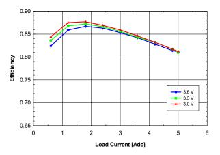
Fig. 0.7525V.4: Efficiency vs. load current and input voltage for Vout = 0.7525 V converter mounted vertically with air flowing from pin 5 to pin 1 at a rate of 200 LFM (1 m/s) and Ta =  $25\,^{\circ}$ C.
