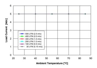
Fig. 1.0V.2: Available load current vs. ambient temperature and airflow rates for Vout = 1.0 V converter mounted horizontally with Vin = 5 V, air flowing from pin 5 to pin 1, and maximum MOSFET temperature  $\leq$  120 °C.
