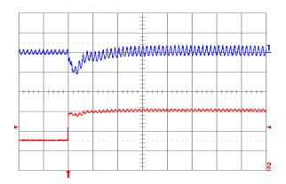
Fig. 1.2V.6: Output voltage response for Vout = 1.2 V to positive load current step change from 2.5 A to 5 A with slew rate of 5 A/ $\mu$ s at Vin = 5 V. Top trace: output voltage (100 mV/div.); Bottom trace: load current (2 A/div.). Co = 47  $\mu$ F ceramic + 1  $\mu$ F ceramic. Time scale: 20  $\mu$ s/div.
