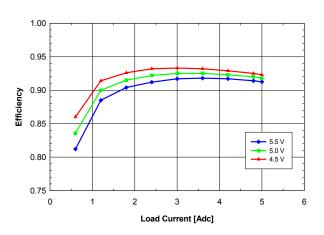
Fig. 2.5V.3: Efficiency vs. load current and input voltage for Vout = 2.5 V converter mounted vertically with air flowing from pin 5 to pin 1 at a rate of 200 LFM (1 m/s) and Ta = 25 °C.
