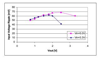
Fig. B: Input Voltage Ripple, C<sub>IN</sub> = 470 μF polymer + 2x47 μF ceramic.
