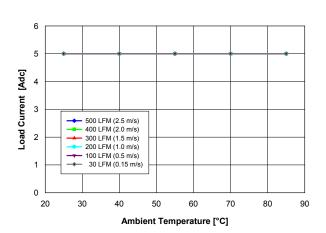
Fig. 1.2V.1: Available load current vs. ambient temperature and airflow rates for Vout = 1.2 V converter mounted vertically with Vin = 5 V, air flowing from pin 5 to pin 1, and maximum MOSFET temperature ≤ 120 °C.
