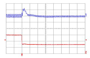
Fig. 1.8V.8: Output voltage response for Vout = 1.8 V to negative load current step change from 5 A to 2.5 A with slew rate of -5 A/ $\mu$ s at Vin = 5 V. Top trace: output voltage (100 mV/div.); Bottom trace: load current (2 A/div.). Co = 47  $\mu$ F ceramic + 1  $\mu$ F ceramic. Time scale: 20  $\mu$ s/div.
