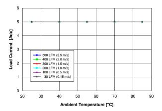
Fig. 1.0V.1: Available load current vs. ambient temperature and airflow rates for Vout = 1.0 V converter mounted vertically with Vin = 5 V, air flowing from pin 5 to pin 1, and maximum MOSFET temperature  $\leq$  120 °C.
