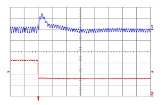
Fig. 3.3V.8: Output voltage response for Vout = 3.3 V to negative load current step change from 5 A to 2.5 A with slew rate of -5 A/ $\mu$ s at Vin = 5 V. Top trace: output voltage (100 mV/div.); Bottom trace: load current (2 A/div.). Co = 47  $\mu$ F ceramic + 1  $\mu$ F ceramic. Time scale: 20  $\mu$ s/div.
