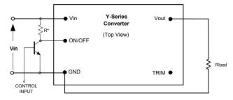
Fig. C: Circuit configuration for ON/OFF function.
