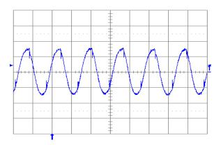
Fig. 2.0V.6: Output voltage ripple (20 mV/div.) at full rated load current into a resistive load with external capacitance 10  $\mu$ F ceramic + 1  $\mu$ F ceramic and Vin = 5 V for Vout = 2.0 V. Time scale: 2  $\mu$ s/div.
