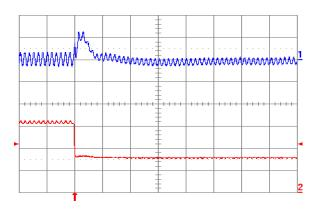
Fig. 2.0V.8: Output voltage response for Vout = 2.0 V to negative load current step change from 5 A to 2.5 A with slew rate of -5 A/ $\mu$ s at Vin = 5 V. Top trace: output voltage (100 mV/div.); Bottom trace: load current (2 A/div.). Co = 47  $\mu$ F ceramic + 1  $\mu$ F ceramic. Time scale: 20  $\mu$ s/div.
