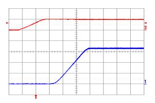
Fig. 3.3V.5: Turn-on transient for Vout = 3.3 V with application of Vin at full rated load current (resistive) and 47 µF external capacitance at Vin = 5 V. Top trace: Vin (5 V/div.); Bottom trace: output voltage (1 V/div.); Time scale: 2 ms/div.
