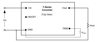
Fig. D: Configuration for programming output voltage.
