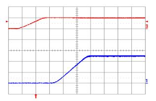
Fig. 2.5V.4: Turn-on transient for Vout = 2.5 V with application of Vin at full rated load current (resistive) and 47 µF external capacitance at Vin = 5 V. Top trace: Vin (5 V/div.); Bottom trace: output voltage (1V/div.); Time scale: 2 ms/div.
