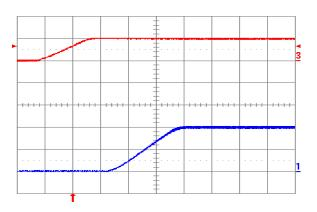
Fig. 2.0V.5: Turn-on transient for Vout = 2.0 V with application of Vin at full rated load current (resistive) and 47  $\mu$ F external capacitance at Vin = 5 V. Top trace: Vin (5 V/div.); Bottom trace: output voltage (1 V/div.); Time scale: 2 ms/div.
