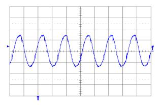
Fig. 1.8V.6: Output voltage ripple (20 mV/div.) at full rated load current into a resistive load with external capacitance 10  $\mu$ F ceramic + 1  $\mu$ F ceramic and Vin = 5 V for Vout = 1.8 V. Time scale: 2  $\mu$ s/div.
