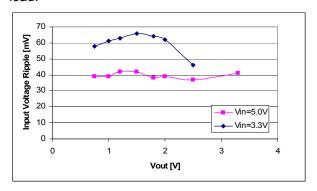
Fig. A: Input Voltage Ripple, C<sub>IN</sub> = 4x47 μF ceramic.
