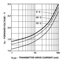
Figure 3. Typical forward voltage vs. drive current.
