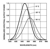
Figure 2. Typical spectra normalized to the 25°C peak.
