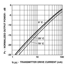
Figure 4. Typical normalized output optical power vs. drive current.
