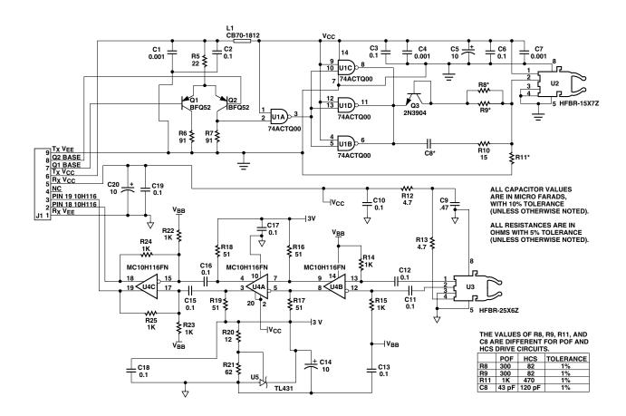
Figure 1. Transmitter and receiver application circuit with  $+5\,\mathrm{V}$  ECL inputs and outputs.
