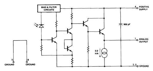
Figure 2. Simplified receiver schematic.
