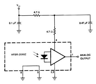
Figure 1. Recommended power supply filter circuit.
