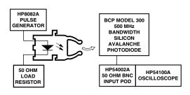
Figure 1. Test circuit for measuring unpeaked rise and fall times.
