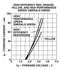
Figure 2. Forward current vs. forward voltage characteristics.
