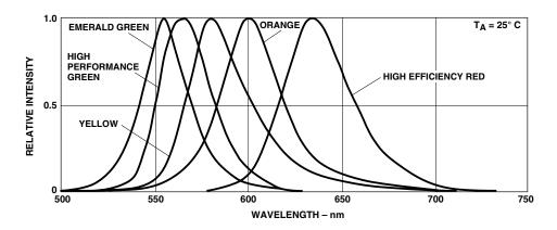
Figure 1. Relative intensity vs. wavelength.
