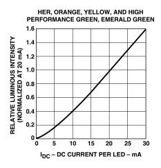
Figure 3. Relative luminous intensity vs. DC forward current.
