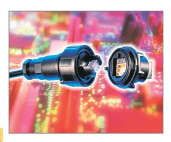
Shroud for RJ45 provides Coupling ring, screw thread protection against damage provides secure cable coupling through mis-use and positive alignment for mating of connectors Panel gasket maintains IP seal to panel Sealing gland and cage optimised to maintain IP seal and provide secure cable restraint without disrupting signal 'O' ring maintains IP seal at Shielded Cat 5e coupler connector interface maintains screening
