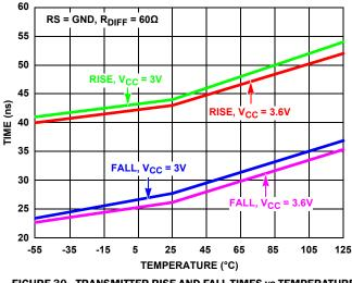
FIGURE 30. TRANSMITTER RISE AND FALL TIMES vs TEMPERATURE AT FAST SPEED
