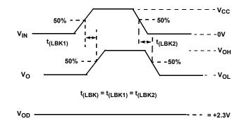
FIGURE 18B. LOOP BACK DELAY TO DOMINANT MEASUREMENT POINTS
