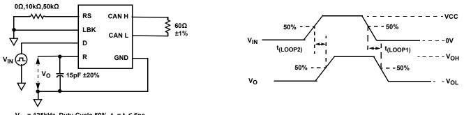
$V_{IN}$  = 125kHz, Duty Cycle 50%,  $t_r = t_f \le 6ns$ .
