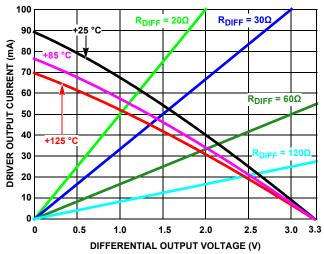
FIGURE 33. DRIVER OUTPUT CURRENT vs DIFFERENTIAL OUTPUT VOLTAGE
