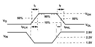
FIGURE 14A. RECEIVER VOLTAGE DEFINITIONS
