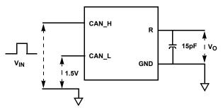
$V_{IN}$  = 125kHz, Duty Cycle 50%, t<sub>r</sub> = t<sub>f</sub> = 6ns, Z<sub>O</sub> = 50 $\Omega$ C<sub>L</sub> includes test setup capacitance
