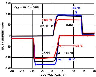
FIGURE 34. DRIVER OUTPUT CURRENT vs SHORT CIRCUIT VOLTAGE vs TEMPERATURE
