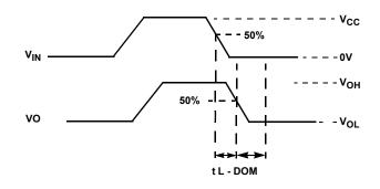
$V_{IN}$  = 125kHz, 0V to  $V_{CC}$ , Duty Cycle 50%,  $t_r = t_f \le 6ns$
