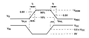
$V_{IN}$  = 125kHz, 0V to  $V_{CC}$ , Duty Cycle 50%,  $t_r$  =  $t_f$   $\leq$  6ns,  $Z_O$  = 50 $\Omega$  C<sub>L</sub> includes fixture and instrumentation capacitance.
