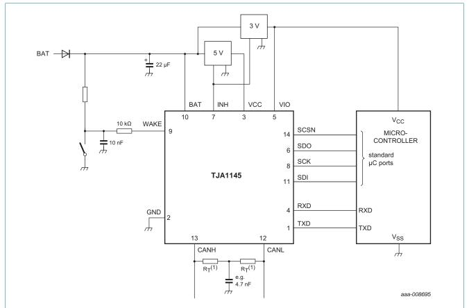
(1) For bus line end nodes,  $R_T = 60~\Omega$  in order to support the 'split termination concept'. For sub-nodes, an optional 'weak' termination of e.g.  $R_T = 1.3~\text{k}\Omega$  can be used, if required by the OEM.
