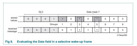
Optionally, the data length code and the data field can be excluded from the evaluation of the wake-up frame. If bit PNDM = 0, only the identifier field is evaluated to determine if the frame contains a valid wake-up message. If PNDM = 1 (the default value), the data field is included as part of the wake-up filtering.
