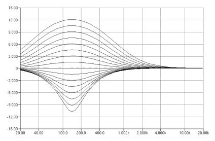
Figure 16: Equaliser filter Band 2 frequency response at FS = 48 kHz
