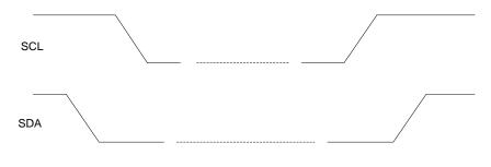
Figure 21 Timing of I2C START and STOP Conditions
