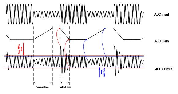
Figure 9: Principle of Operation of the ALC
