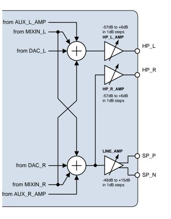
Figure 11: Analogue output signal paths and gain ranges
