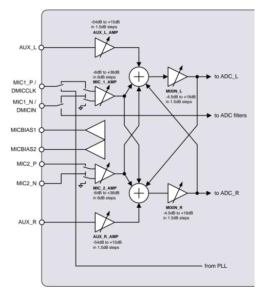
Figure 6: Audio input routing and gain ranges
