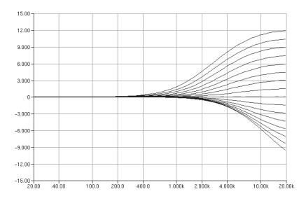
Figure 19: Equaliser filter Band 5 frequency response at FS = 48 kHz
