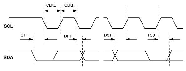
Figure 4: I2C Bus Timing
