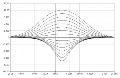
Figure 17: Equaliser filter Band 3 frequency response at FS = 48 kHz
