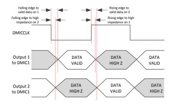
Figure 8: Digital microphone timing example
