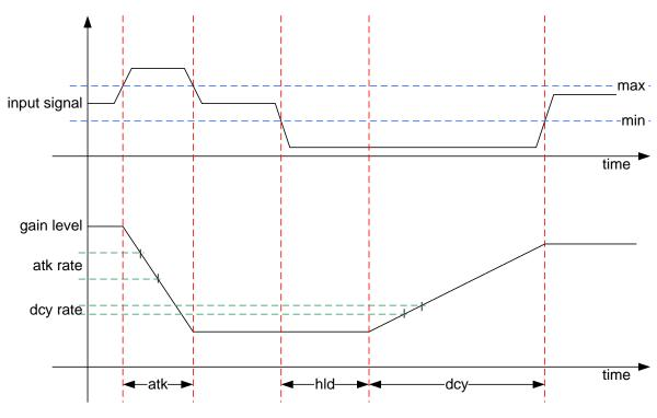
Figure 10: Attack, Delay and Hold parameters
