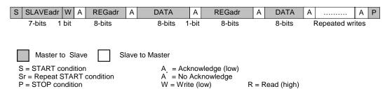
Figure 29: 2-WIRE Repeated Write (SDA Line)
