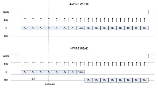
Figure 23: 4-WIRE Host Write and Read Ttiming (nCS\_POL = '0', CPOL = '1', CPHA = '1')
