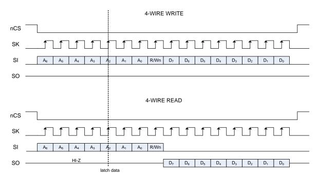
Figure 20: 4-WIRE Host Write and Read Timing (nCS\_POL = '0', CPOL = '0', CPHA = '0')
