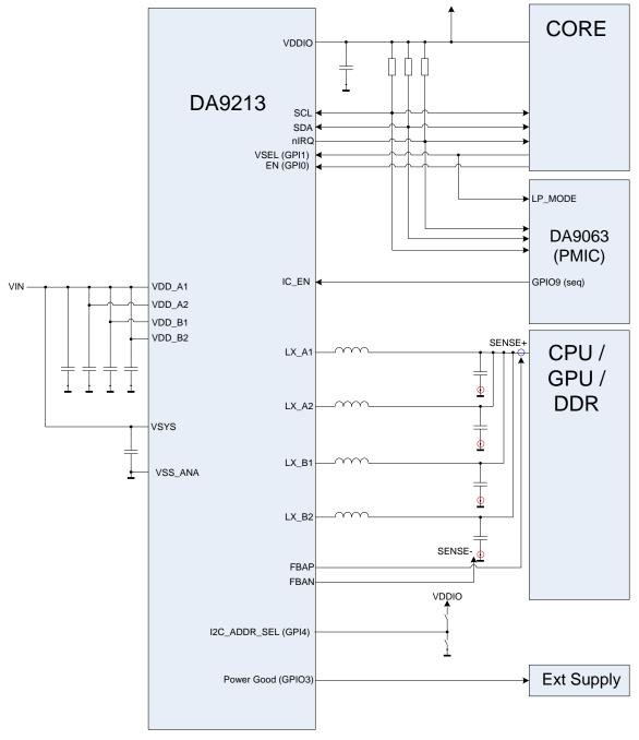
Figure 14: Typical Application of DA9213
