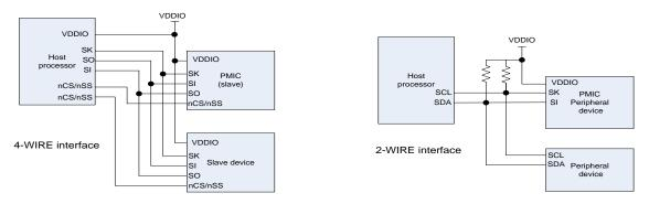
Figure 19: Schematic of 4-WIRE and 2-WIRE Power Manager Bus
