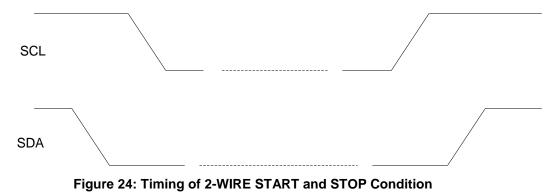
The 2-WIRE bus is monitored by DA9213, DA9214, and DA9215 for a valid SLAVE address whenever the interface is enabled. It responds immediately when it receives its own slave address. The acknowledge is done by pulling the SDA line low during the following clock cycle (white blocks marked with 'A' in Figure 25 to Figure 29).
