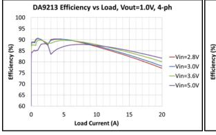
Figure 9: 4 Phase Auto-Mode, 0 to 20 A (Linear)
