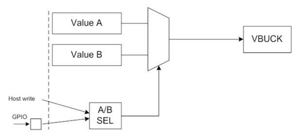
Figure 16: Concept of Control of the Buck's Output Voltage
