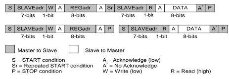
Figure 26: Examples of 2-WIRE Byte Read (SDA Line)
