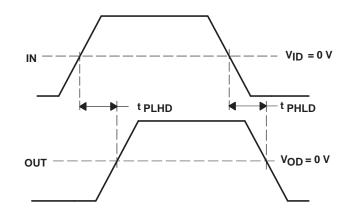
Figure 6. Propagation Delay Input to Output
