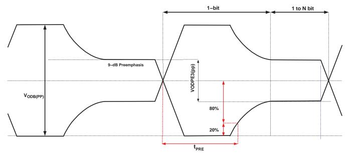
Figure 4. t<sub>(PRE</sub>) Preemphasis Duration Measurement
