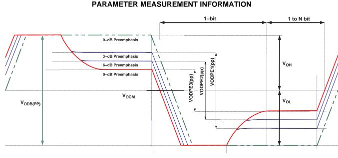
Figure 3. Preemphasis and Output Voltage Waveforms and Definitions
