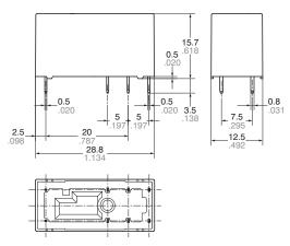
**Dimension: Tolerance** ±0.1±.004 Less than 1 mm.039inch: Min. 1 mm.039inch less than 3 mm.118inch: ±0.2±.008 Min. 3 mm.118inch: ±0.3±.012
