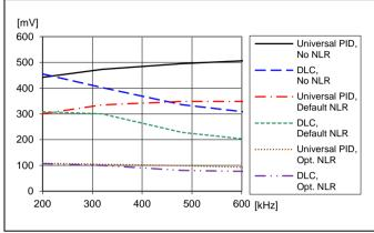
Load transient peak voltage deviation vs. frequency. Step-change (12.5-37.5-12.5 A).  $T_{P1} = +25 \, ^{\circ}\text{C}, \, V_{I} = 12 \, \text{V}, \, V_{O} = 1.0 \, \text{V}, \, C_{O} = 470 \, \mu\text{F}/10 \, \text{m}\Omega$
