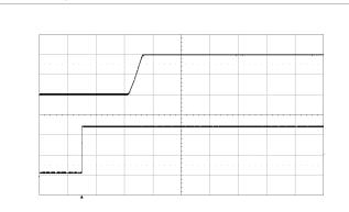
Start-up enabled by connecting V<sub>I</sub> at:  $T_{P1} = +25^{\circ}C$ , V<sub>I</sub> = 12 V, V<sub>O</sub> = 1.0 V  $C_{O} = 470 \ \mu\text{F}/10 \ \text{m}\Omega$ , I<sub>O</sub> = 40 A
