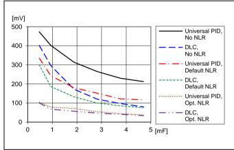
Load transient peak voltage deviation vs. decoupling capacitance. Step (12.5-37.5-12.5 A). Parallel coupling of capacitors with 470  $\mu F/10$  m $\Omega,$  $T_{P1} = +25 \, ^{\circ}\text{C}. \, V_{I} = 12 \, \text{V}, \, V_{O} = 1.0 \, \text{V}, \, f_{sw} = 320 \, \text{kHz}, \, \text{di/dt} = 2 \, \text{A/µs}$
