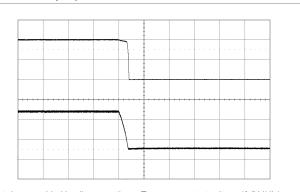
Shut-down enabled by disconnecting V<sub>1</sub> at:  $T_{P1} = +25~^{\circ}\text{C}, \text{V}_{1} = 12~\text{V}, \text{V}_{O} = 1.0~\text{V}$   $C_{O} = 470~\mu\text{F}/10~\text{m}\Omega, \text{I}_{O} = 50~\text{A}$
