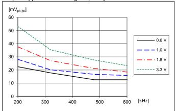
Output voltage ripple  $V_{pk-pk}$  at:  $T_{P1}$  = +25 °C,  $V_I$  = 12 V,  $C_O$  = 470  $\mu$ F/10  $m\Omega$ ,  $I_0$  = 50 A resistive load. Default configuration except changed frequency.
