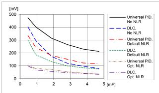
Load transient peak voltage deviation vs. external capacitance. Step (12.5-37.5-12.5 A). Parallel coupling of capacitors with 470  $\mu$ F/10 m $\Omega$ ,  $T_{P1}$  = +25 °C.  $V_1$ = 12 V,  $V_0$ = 1.0 V,  $f_{sw}$ = 320 kHz, di/dt = 2 A/ $\mu$ s
