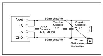
Output ripple and noise test set-up.
