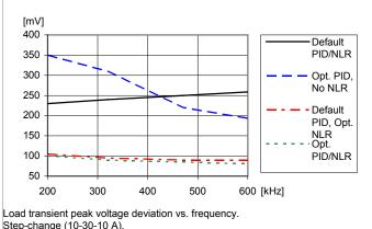
Step-change (10-30-10 A).  $T_{P1}$  = +25°C.  $V_i$ =12 V,  $V_O$ =1.0 V,  $C_O$ =470  $\mu$ F/10 m $\Omega$
