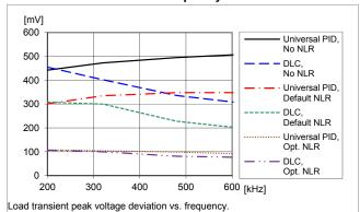
Step-change (12.5-37.5-12.5 A).  $T_{P1}$  = +25 °C.  $V_1$  = 12 V,  $V_0$  = 1.0 V,  $C_0$  = 470  $\mu$ F/10 m $\Omega$
