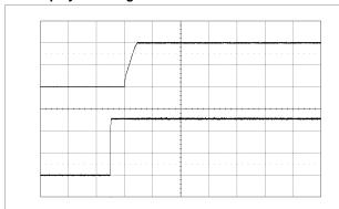
Start-up by enabling CTRL signal at: T  $_{P1}$  = +25 °C, V  $_{I}$  = 12 V, V  $_{O}$  = 1.0 V C  $_{O}$  = 470  $\mu F/10$  m $\Omega,\ I_{O}$  = 50 A
