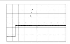
Start-up enabled by connecting V<sub>I</sub> at:  $T_{P1}$  = +25 °C, V<sub>I</sub> = 12 V, V<sub>O</sub> = 1.0 V  $C_O$  = 470  $\mu$ F/10 m $\Omega$ , I $_O$  = 50 A
