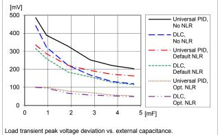
Load transient peak voltage deviation vs. external capacitance. Step (12.5-37.5-12.5 A). Parallel coupling of capacitors with 470  $\mu\text{F}/10$  m $\Omega$ , T  $_{\text{P1}}$  = +25 °C. V  $_{\text{I}}$  = 12 V, V  $_{\text{O}}$  = 3.3 V, f  $_{\text{sw}}$  = 320 kHz, di/dt = 2 A/ $\mu\text{s}$
