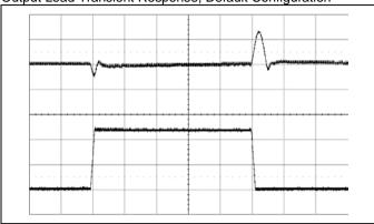
Output voltage response to load current stepchange (12.5-37.5-12.5 A) at: Top trace: output voltage (200 mV/div.). Bottom trace: load current (10 A/div.). Time scale: (0.1 ms/div.). di/dt=2 A/ $\mu$ S,  $f_{sw}=320$  kHz,  $C_{O}=470$  µF/10 m $\Omega$  Default configuration (DLC and default NLR)
