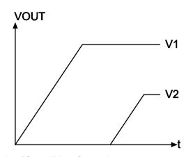
Illustration of Output Voltage Sequencing.
