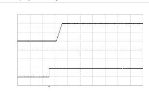
Start-up by enabling CTRL signal at:  $T_{P1}$  = +25°C,  $V_{I}$  = 12 V,  $V_{O}$  = 1.0 V  $C_{O}$  = 470  $\mu$ F/10 m $\Omega$ ,  $I_{O}$  = 40 A
