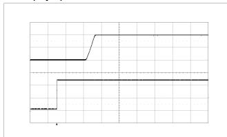
Start-up enabled by connecting V<sub>I</sub> at:  $T_{P1}$  = +25°C, V<sub>I</sub> = 12 V, V<sub>O</sub> = 1.0 V C<sub>O</sub> = 470  $\mu$ F/10 m $\Omega$ , I<sub>O</sub> = 40 A
