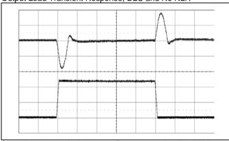
Output voltage response to load current step-change (12.5-37.5-12.5 A) at:  $T_{\rm P,I} = +25~{\rm ^C}, V_{\rm I} = 12~V, V_{\rm O} = 1.0~V \\ {\rm d}/{\rm dt} = 2~{\rm A/ps}, f_{\rm sw} = 320~{\rm kHz}, C_{\rm O} = 470~{\rm \mu F/10~m}\Omega$  DLC and no NLR
