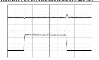
Output voltage response to load current step-Output voltage leaponise of loss of size of section change (12.5-37.5-12.5 A) at:  $T_{P1} = +25 \, ^{\circ}\text{C}, \, V_{I} = 12 \, \text{V}, \, V_{O} = 1.0 \, \text{V}$  di/dt=2 A/µs,  $f_{sw} = 320 \, \text{kHz}, \, C_{O} = 470 \, \mu\text{F}/10 \, \text{m}\Omega$ DLC and optimized NLR
