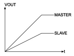
Illustration of Ratiometric Voltage Tracking
