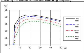
Efficiency vs. load current and switching frequency at  $T_{P1} = +25 \,^{\circ}\text{C}, V_{I} = 12 \,\text{V}, V_{O} = 1.0 \,\text{V}, C_{O} = 470 \,\mu\text{F}/10 \,\text{m}\Omega$ Default configuration except changed frequency
