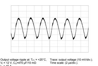
$V_1 = 12 \text{ V}, C_0 = 470 \mu\text{F}/10 \text{ m}\Omega$  $I_0 = 40 \text{ A}$
