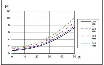
Dissipated power vs. load current and switching frequency at  $T_{P1}$  = 25 °C, V<sub>I</sub>= 12 V, V<sub>O</sub>= 1.0 V, C<sub>O</sub>= 470  $\mu F/10$  m $\Omega$  Default configuration except changed frequency
