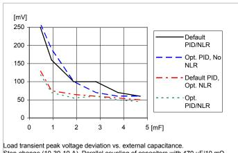
Step-change (10-30-10 A). Parallel coupling of capacitors with 470  $\mu$ F/10 m $\Omega$ , T<sub>P1</sub> = +25°C. V<sub>I</sub>=12 V, V<sub>O</sub>=1.0 V, f<sub>sw</sub>=320 kHz, di/dt=2 A/ $\mu$ s
