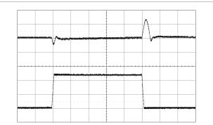
Output voltage response to load Step-change (12.5-37.5-12.5 A) at:  $T_{P1} = +25\,^{\circ}\mathrm{C},\ V_{1} = 12\ V,\ V_{0} = 1.0\ V$  di/dt = 2 A/µs,  $f_{s_{N}} = 320\ kHz$   $C_{0} = 470\ \mu F/10\ m\Omega$
