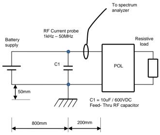
Conducted EMI test set-up
