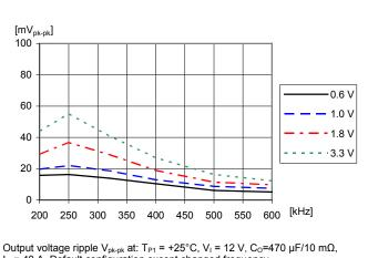
Output voltage ripple V<sub>pk-pk</sub> at: T<sub>P1</sub> = +25°C, V<sub>I</sub> = 12 V, C<sub>O</sub>=470  $\mu$ F/10 m $\Omega$ , I<sub>O</sub> = 40 A. Default configuration except changed frequency.
