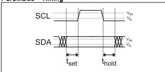
Setup and hold times timing diagram
