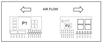
Temperature positions and air flow direction.
