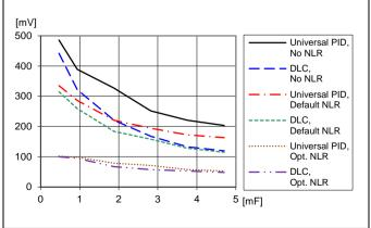
Load transient peak voltage deviation vs. decoupling capacitance. Step (12.5-37.5-12.5 A). Parallel coupling of capacitors with 470  $\mu F/10$  m $\Omega,$  $T_{P1} = +25 \, ^{\circ}\text{C}. \, V_{I} = 12 \, V, \, V_{O} = 3.3 \, V, \, f_{sw} = 320 \, kHz, \, di/dt = 2 \, A/\mu s$
