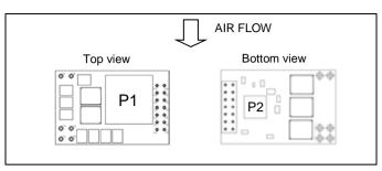
Temperature positions and air flow direction.
