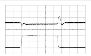
Output voltage response to load current step-change (10-30-10 A) at:  $T_{P1} = +25^{\circ}C$ ,  $V_{I} = 12$  V,  $V_{O} = 1.0$  V di/dt=2 A/ $\mu$ s,  $f_{sw}$ =320 kHz,  $C_{O}$ =470  $\mu$ F/10 m $\Omega$
