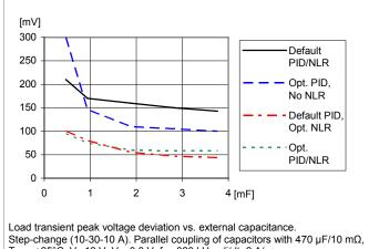
Step-change (10-30-10 A). Parallel coupling of capacitors with 470  $\mu$ F/10 m $\Omega$ , T<sub>P1</sub> = +25°C. V<sub>I</sub>=12 V, V<sub>O</sub>=3.3 V, f<sub>sw</sub>=320 kHz, di/dt=2 A/ $\mu$ s
