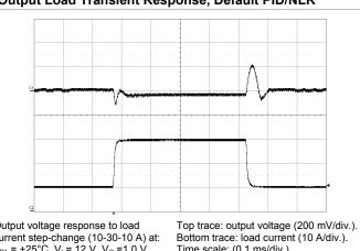
Output voltage response to load current step-change (10-30-10 A) at:  $T_{P1}$  = +25°C,  $V_{I}$  = 12 V,  $V_{O}$  =1.0 V di/dt=2 A/µs,  $f_{sw}$ =320 kHz,  $C_{O}$ =470 µF/10 m $\Omega$  Time scale: (0.1 ms/div.).
