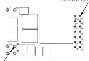
$\acute{\text{P}}\text{in}$  2B for measurement of minimum Pin (solder joint) temperature  $T_{\text{PIN}}$
