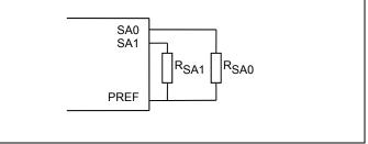
Schematic of connection of address resistor.
