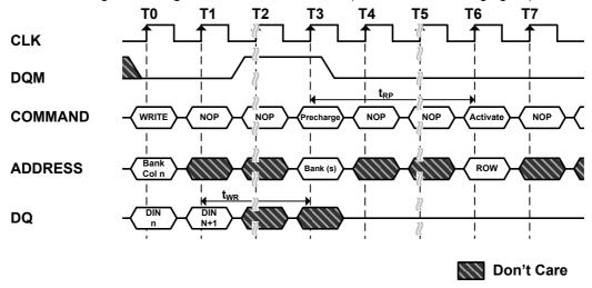
Note: The LDQM/UDQM can remain low in this example if the length of the write burst is 1 or 2.
