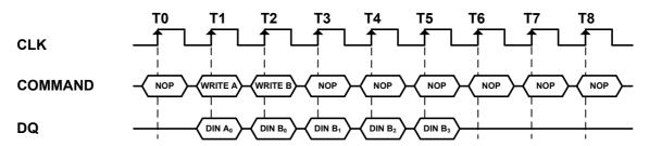
Figure 11. Write Interrupted by a Write (Burst Length = 4)
