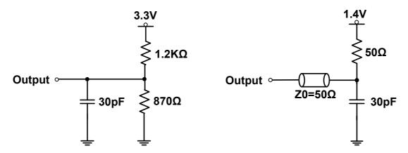
Figure 18.1 LVTTL D.C. Test Load (A)
