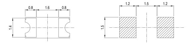
**Note:** Tolerances Unless Dimension  $\pm 0.1$ mm, Unit = mm
