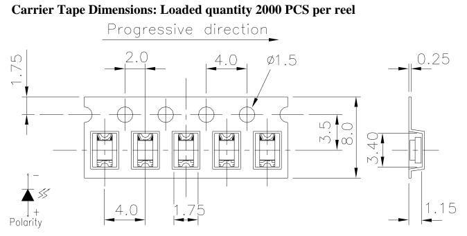
**Note:** Tolerances Unless Dimension  $\pm 0.1$ mm, Unit = mm
