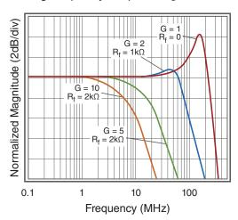
Non-Inverting Frequency Response  $V_S = +2.7V$
