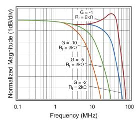
Inverting Frequency Response  $V_S = +2.7V$
