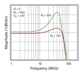
Figure 5: Frequency Response vs. Rf
