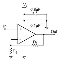
Figure 4: Single Supply Non-Inverting Gain Circuit
