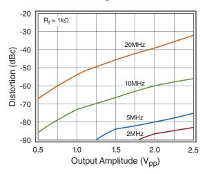
$T_A = 25$ °C,  $V_S = +5V$ ,  $R_L = 2k\Omega$  to  $V_S/2$ , G = +2,  $R_F = 2k\Omega$ ; unless otherwise noted.
