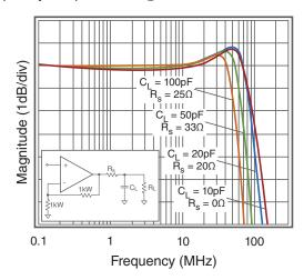
Inverting Frequency Response  $V_S = +5V$
