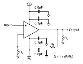
Figure 1: Typical Non-Inverting Gain Circuit
