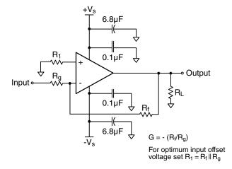
Figure 2: Typical Inverting Gain Circuit
