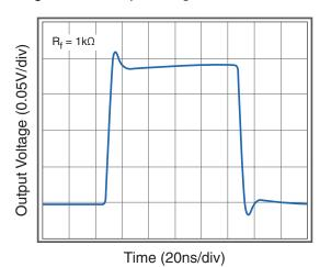
$T_A = 25$ °C,  $V_S = +5V$ ,  $R_L = 2k\Omega$  to  $V_S/2$ , G = +2,  $R_F = 2k\Omega$ ; unless otherwise noted.
