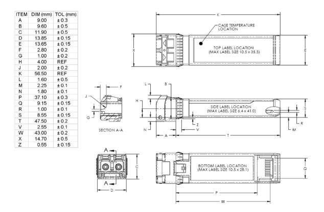
Figure 2. Mechanical Dimensions
