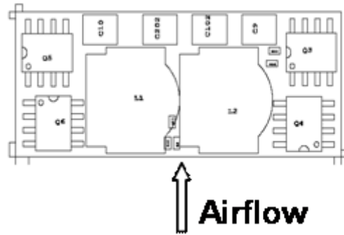
Figure 34. Airflow direction for thermal testing.
