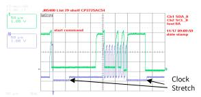
Example waveforms showing clock stretching.
