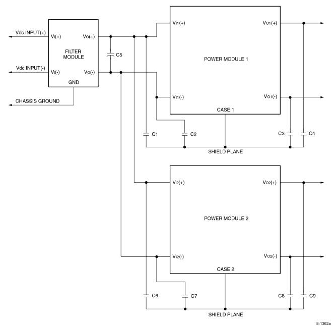
Note: C1 through C4 and C6 through C9 can be 0.01 µF to 0.1 µF. Select the voltage rating to meet input-to-output isolation requirements. C5 should be the recommended value indicated in the power module data sheet.
