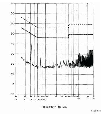
Figure 10. JW075A5 Conducted Noise with Filter
