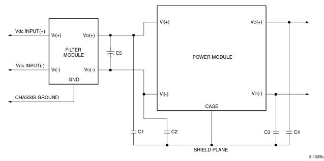
Note: C1 through C4 can be 0.01 μF to 0.1 μF. Select the voltage rating to meet input-to-output isolation requirements. C5 should be the recommended value indicated in the power module data sheet.
