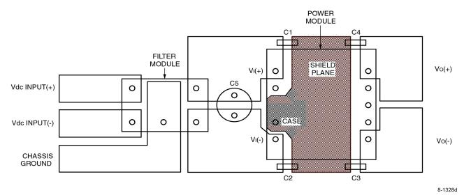
Note: Vdc input(+) and Vdc input(-) planes should overlay each other, as should the VI(+) and VI(-) planes, as should the VO(+) and VO(-) planes. Avoid routing signals or planes under the power module or the filter module. Ensure all connections are low impedance.
