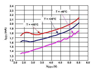
FIGURE 11. I<sub>CC1</sub> ENABLED CURRENT vs V<sub>CC1</sub> (ISL33001)
