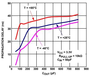
FIGURE 24. PROPAGATION DELAY H-L vs Cout
