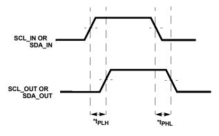
\*Propagation delay measured between 50% of  $V_{\mbox{\scriptsize CC1}}$
