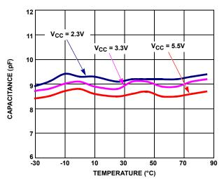
FIGURE 25. SDA/SCL PIN CAPACITANCE vs TEMPERATURE vs  $V_{CC}$
