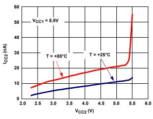
FIGURE 16. I<sub>CC2</sub> DISABLED CURRENT vs V<sub>CC2</sub> (ISL33003)
