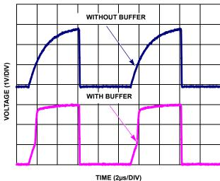
FIGURE 2. BUS ACCELERATOR PERFORMANCE
