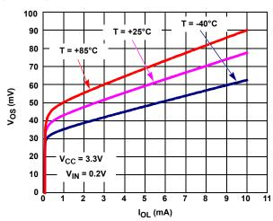
FIGURE 20. INPUT TO OUTPUT OFFSET VOLTAGE VS SINK CURRENT VS TEMPERATURE
