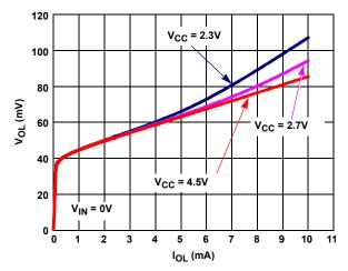
FIGURE 17. SDA/SCL OUTPUT LOW VOLTAGE vs SINK CURRENT vs  $V_{\mbox{\scriptsize CC}}$
