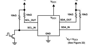
FIGURE 8. ACCELERATOR CURRENT TEST CIRCUIT
