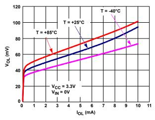
FIGURE 18. SDA/SCL OUTPUT LOW VOLTAGE vs SINK CURRENT vs
