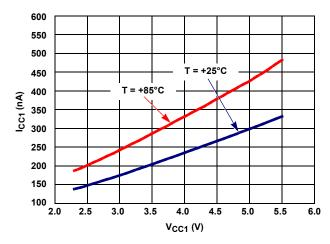
FIGURE 12.  $I_{CC1}$  DISABLED CURRENT vs  $V_{CC1}$  (ISL33001)
