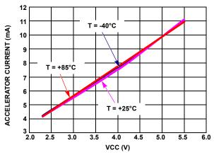
FIGURE 21. ACCELERATOR PULL-UP CURRENT vs V<sub>CC</sub>
