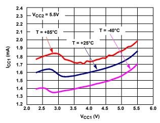
FIGURE 13.  $I_{CC1}$  ENABLED CURRENT vs  $V_{CC1}$  (ISL33002 AND ISL33003)
