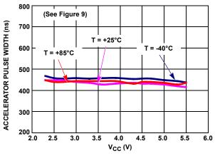
FIGURE 22. ACCELERATOR PULSE WIDTH vs V<sub>CC</sub>
