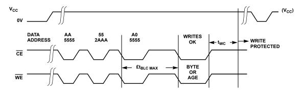
FIGURE 7. TIMING SEQUENCE BYTE OR PAGE WRITE
