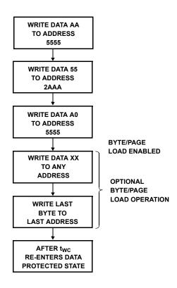
FIGURE 8. WRITE SEQUENCE FOR SOFTWARE DATA **PROTECTION**
