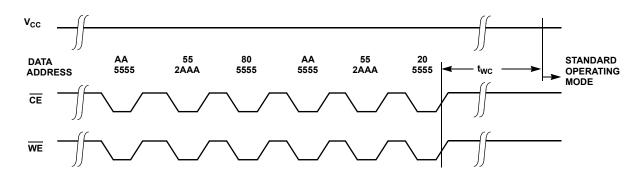
FIGURE 9. RESET SOFTWARE DATA PROTECTION TIMING SEQUENCE
