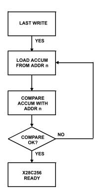
FIGURE 6. TOGGLE BIT SOFTWARE FLOW
