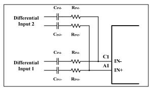
Figure 12 Summing Two Differential Inputs
