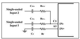
Figure 14 Summing Two Single-Ended Inputs
