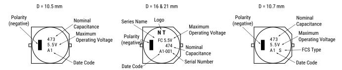
Displays nominal capacitance, maximum operating voltage serial number, polarity, etc.
