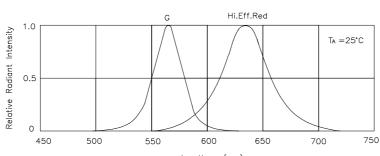
wavelength  $\lambda$  (nm) RELATIVE INTENSITY Vs. WAVELENGTH
