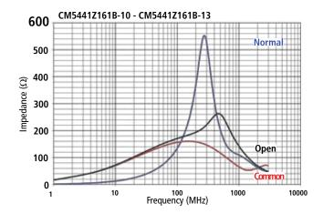
Normal / Differential Mode Impedance: The total impedance to the differential circuit.
