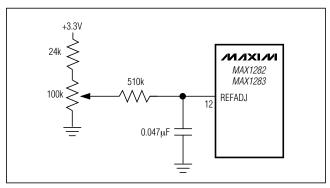
Figure 12. MAX1282/MAX1283 Reference-Adjust Circuit
