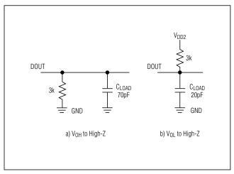
Figure 2. Load Circuits for Disable Time
