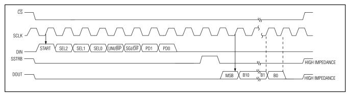
Figure 18. MAX1282/MAX1283-to-TMS320 Serial Interface
