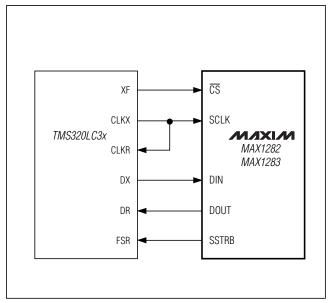
Figure 17. MAX1282/MAX1283-to-TMS320 Serial Interface
