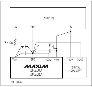
Figure 15. Power-Supply Grounding Connection
