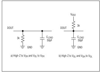
Figure 1. Load Circuits for Enable Time
