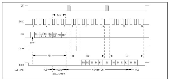
Figure 5. Single-Conversion Timing
