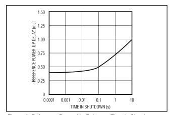
Figure 8. Reference Power-Up Delay vs. Time in Shutdown
