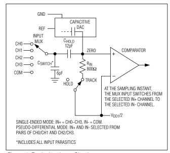
Figure 4. Equivalent Input Circuit
