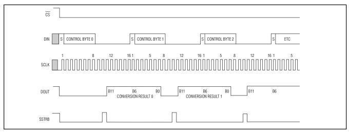
Figure 7. Continuous 16-Clock/Conversion Timing
