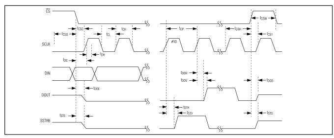
Figure 6. Detailed Serial-Interface Timing
