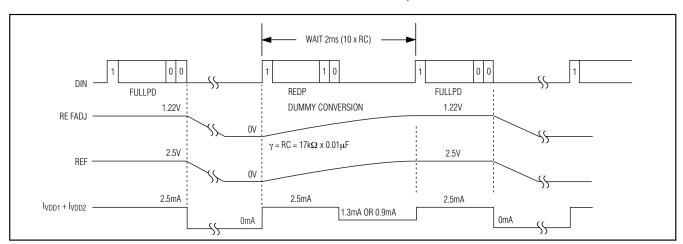
Figure 11a. Full Power-Down Timing
