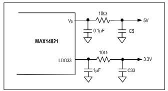
Figure 8. Larger Bypass Capacitance for Powering External Circuits
