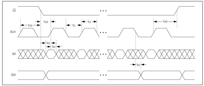
Figure 6. SPI Timing Diagram
