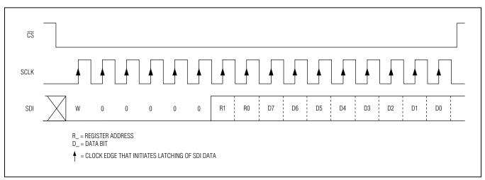
Figure 11. SPI Write Cycle
