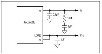
Figure 7. V<sub>5</sub> Compensation Network
