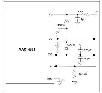
Figure 14. MAX14821 Operating Circuit with TVS Protection
