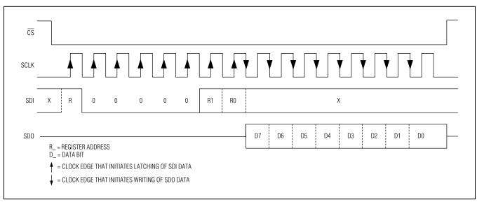
Figure 12. SPI Read Cycle
