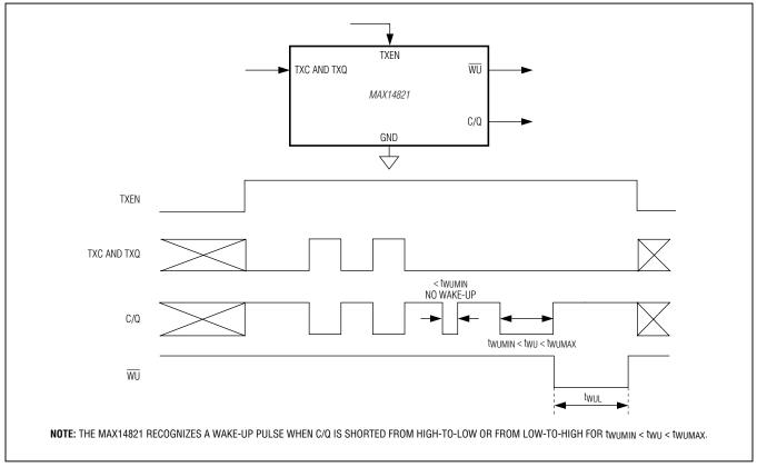
Figure 5. Wake-Up Detection Timing
