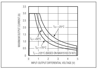
Figure 1. Maximum Output Current Curves
