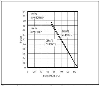
Figure 1. Calculated Maximum Power Dissipation vs. Ambient Temperature
