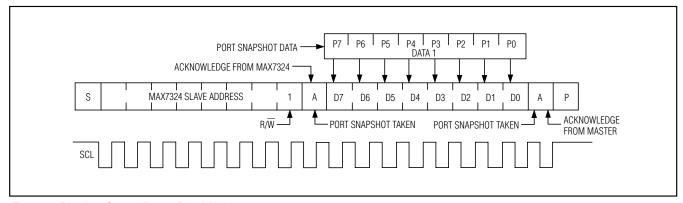
Figure 8. Reading Output Ports of the MAX7324
