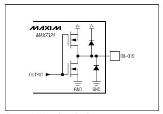
Figure 11. MAX7324 Output Port Structure
