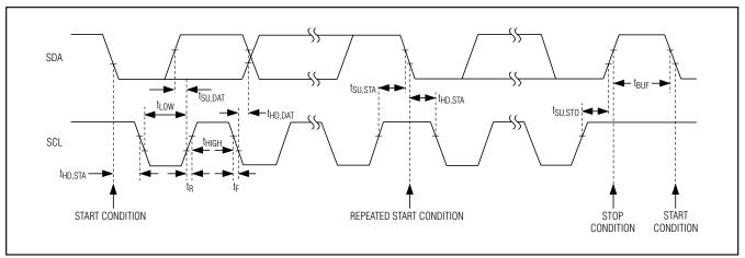
Figure 1. 2-Wire Serial-Interface Timing Details
