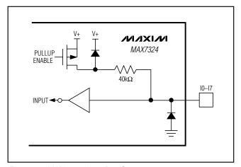
Figure 12. MAX7324 Input Port Structure
