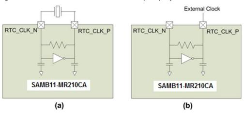
Figure 5-2. SAMB11 XO Connections to Low Frequency Crystal Oscillator
