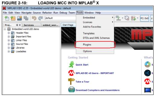
When the Plugins window appears, click on the table for Available Plugins and select MCC from the list of options and click on the **Install** button at the bottom left of the window. The IDE will then download and install the MCC within MPLAB X.
