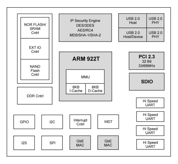
Figure 1. KSZ9692PB Block Diagram
