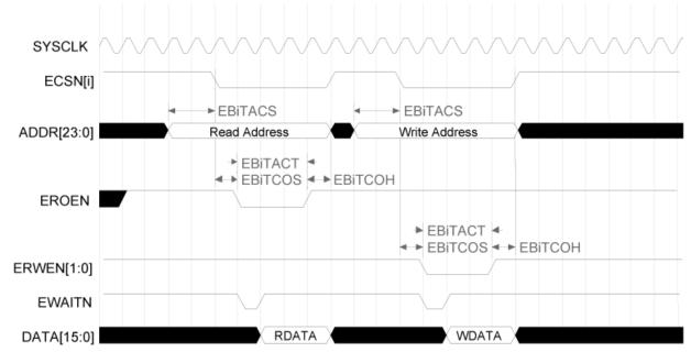
Figure 19 provides external I/O ports interface timing.
