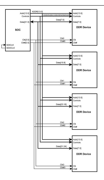
Figure 9. Two 8-bit DDR Memory Devices Interface Example
