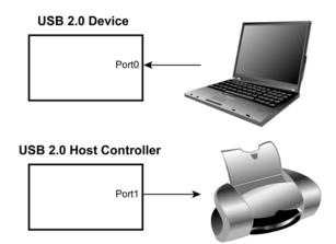
Figure 13. USB 2.0 Configuration as Host + Device
