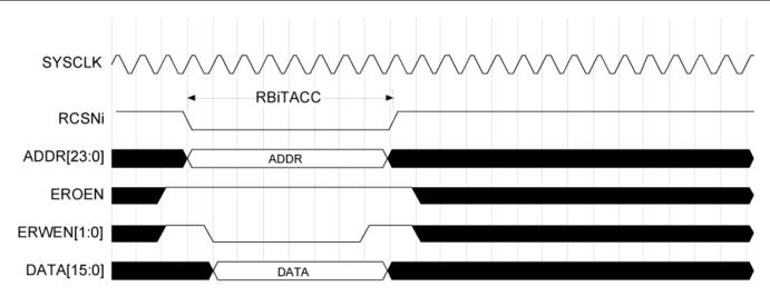
Figure 18. Static Memory Write Cycle
