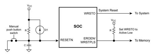
Figure 14. Reset Circuit
