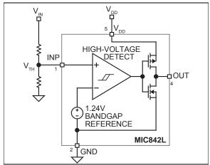
FIGURE 1-5: MIC842L Block Diagram
