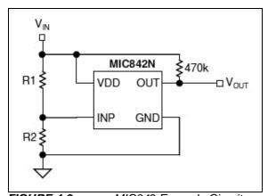
FIGURE 4-3: MIC842 Example Circuit
