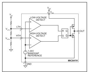
FIGURE 1-1: MIC841H Block Diagram
