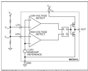
FIGURE 1-2: MIC841L Block Diagram
