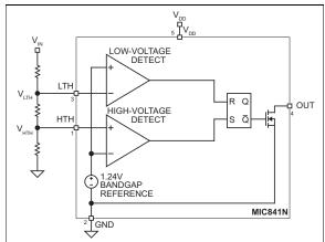
FIGURE 1-3: MIC841N Block Diagram
