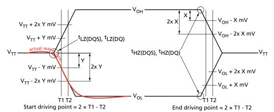
7. Measured from the point when DQS\_t/DQS\_c begins driving the signal, to the point when DQS\_t/DQS\_c begins driving the first rising strobe edge.
