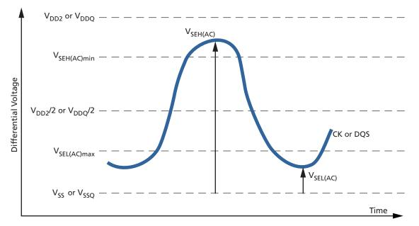
While CA and DQ signal requirements are referenced to  $V_{REF}$ , the single-ended components of differential signals also have a requirement with respect to  $V_{DDO}/2$  for DQS, and  $V_{DD2}/2$  for CK.
