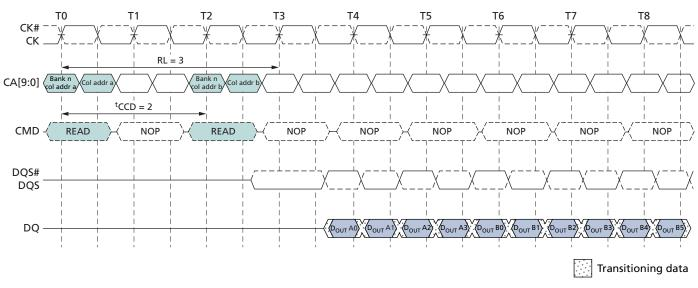
Figure 22: READ Burst Interrupt Example – RL = 3, BL = 8, <sup>t</sup>CCD = 2
