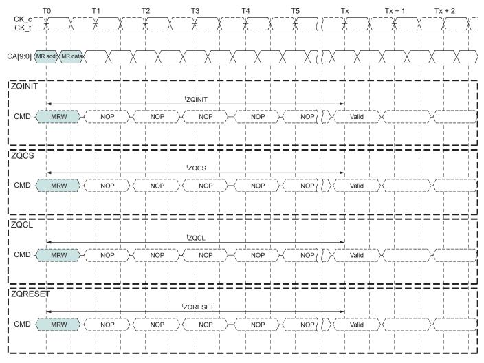
Notes: 1. Only the NOP command is supported during ZQ calibrations <sup>t</sup>ZQINIT: ZQ calibration initialization period <sup>t</sup>ZQCS: ZQ calibration short period <sup>t</sup> ZQCL: ZQ calibration long period <sup>t</sup>ZQRESET: ZQ calibration reset period
