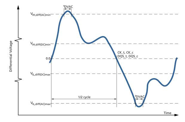
Figure 55: Differential AC Swing Time and <sup>t</sup>DVAC
