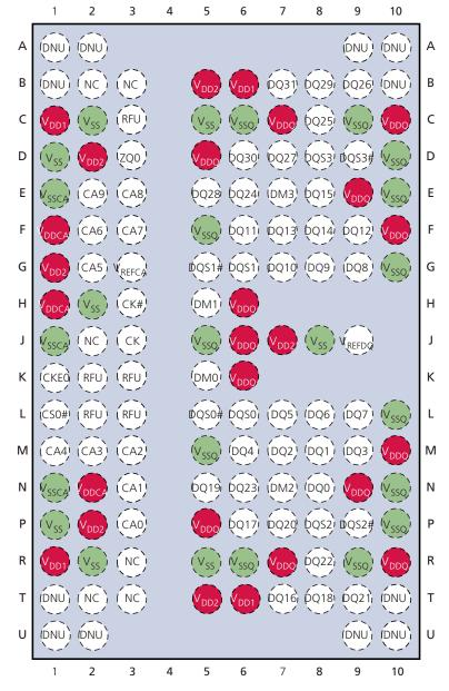
Note: 1. V<sub>DDCA</sub> is unnecessary. F1, H1, N2 pins should be left unconnected.
