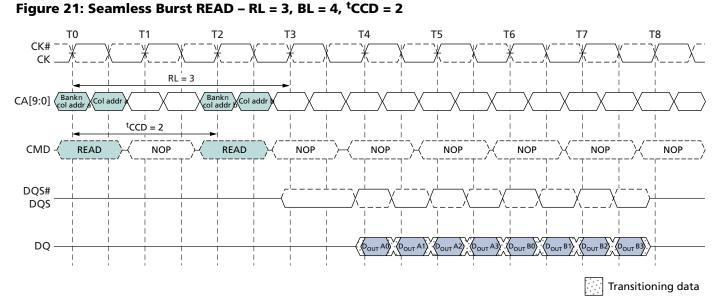
A seamless burst READ operation is supported by enabling a READ command at every other clock cycle for BL = 4 operation, every fourth clock cycle for BL = 8 operation, and every eighth clock cycle for BL = 16 operation. This operation is supported as long as the banks are activated, whether the accesses read the same or different banks.
