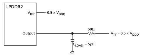
Note: 1. All output timing parameter values (<sup>t</sup>DQSCK, <sup>t</sup>DQSQ, <sup>t</sup>QHS, <sup>t</sup>HZ, <sup>t</sup>RPRE etc.) are reported with respect to this reference load. This reference load is also used to report slew rate.
