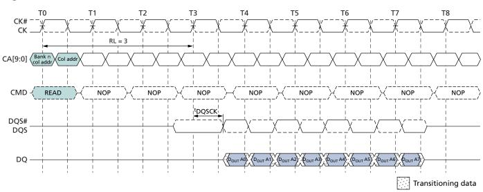
Figure 20: Burst READ – RL = 3, BL = 8, <sup>t</sup>DQSCK < <sup>t</sup>CK
