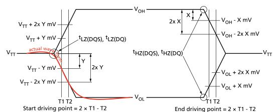
Measured from the point when DQS\_t/DQS\_c begins driving the signal, to the point when DQS\_t/DQS\_c begins driving the first rising strobe edge.
