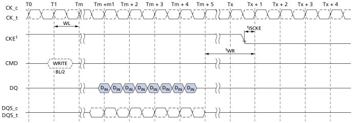
Note: 1. CKE can be registered LOW at (WL + 1 + BL/2 + RU(<sup>t</sup>WR/<sup>t</sup>CK)) clock cycles after the clock on which the WRITE command is registered.
