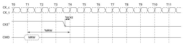
Note: 1. CKE can be registered LOW <sup>t</sup>MRW after the clock on which the MRW command is registered.
