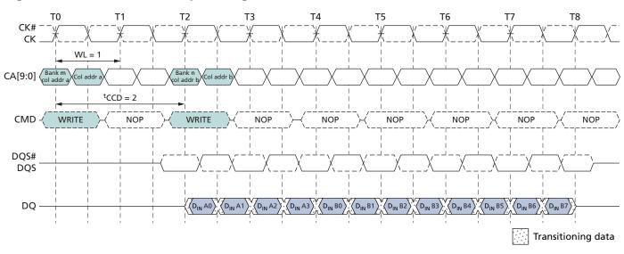
Figure 31: WRITE Burst Interrupt Timing – WL = 1, BL = 8, <sup>t</sup>CCD = 2
