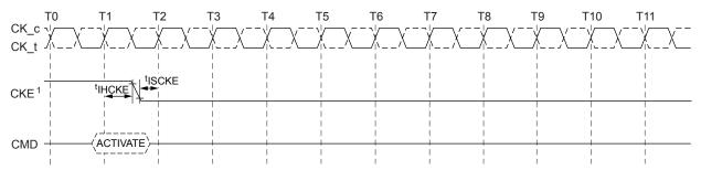
Note: 1. CKE can go LOW at <sup>t</sup>IHCKE after the clock on which the ACTIVATE command is registered.
