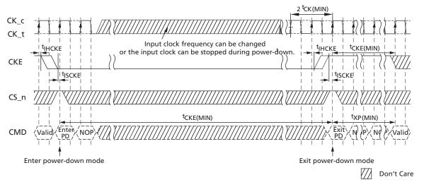
Note: 1. Input clock frequency can be changed or the input clock stopped during power-down, provided that the clock frequency is between the minimum and maximum specified frequencies for the speed grade in use, and that prior to power-down exit, a minimum of two stable clocks complete.
