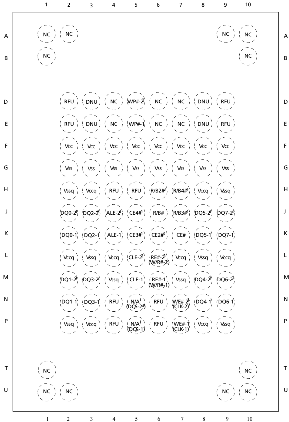
Figure 3: 100-Ball BGA (Ball-Down, Top View)
