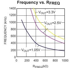
Generally, the NB638 is set for 200 kHz to 1MHz application. It is optimized to operate at high switching frequency with high efficiency. High switching frequency makes it possible to utilize small sized LC filter components to save system PCB space.
