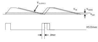
Figure 5—Jitter in Skip Mode
