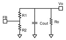
Figure 8—Simplified Circuit in skip Mode
