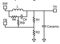
Figure 10—Simplified Circuit of Ceramic Capacitor
