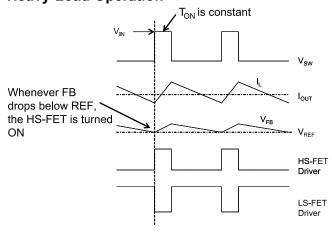
Figure 2—Heavy Load Operation
