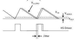
Figure 4—Jitter in PWM Mode
