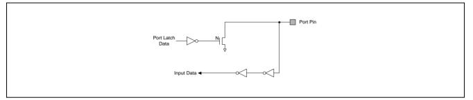
Figure 9-2 Open Drain Output
