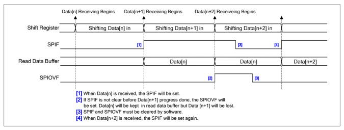
Figure 13–7 SPI Overrun Waveform
