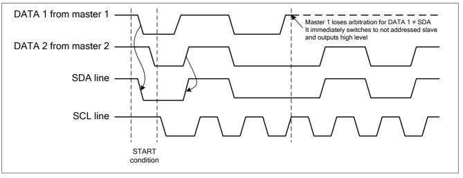
Figure 16-6 Arbitration Procedure of Two Masters
