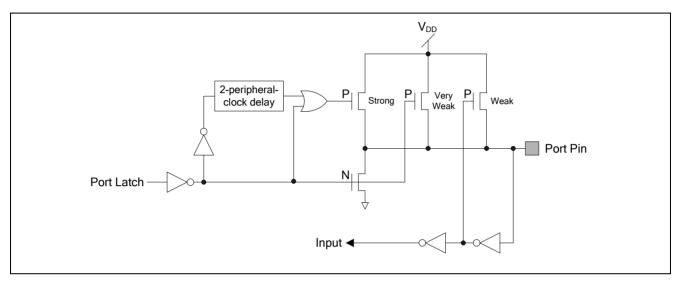
Figure 9-1 Quasi Bi-direction I/O Structure
