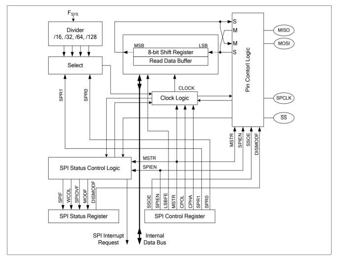
Figure 13–1 SPI Block Diagram
