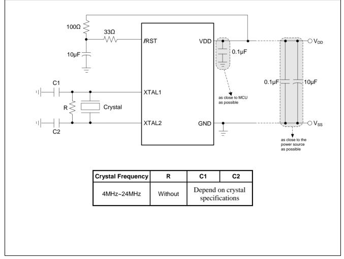
Figure 29–1 Application Circuit for EFT Improvement
