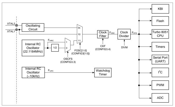
Figure 22–1 Clock System Block Diagram
