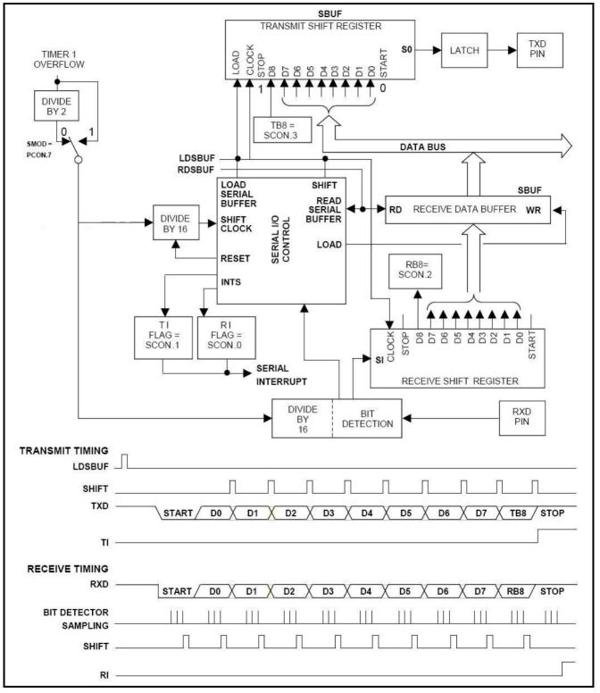
Figure 12–5 Serial Port Mode 3 Function Block
