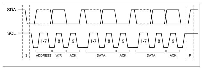
Figure 16–4 Data Format of I<sup>2</sup>C Transfer
