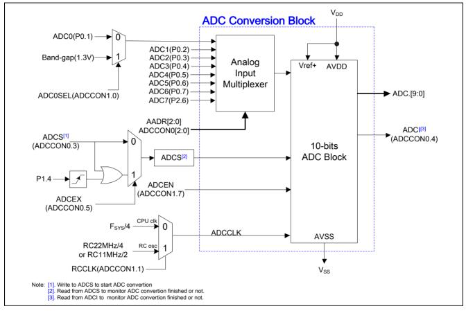
Figure 15-2 ADC Block Diagram
