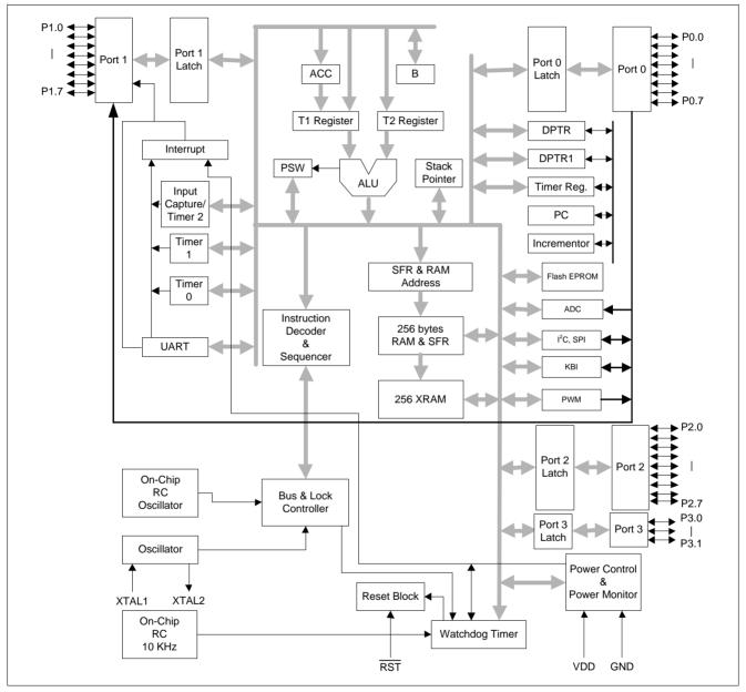
Figure 4–1 N79E855A/854A Function Block Diagram
