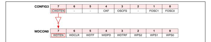
Figure 25–4 CONFIG3 Reset Reloading
