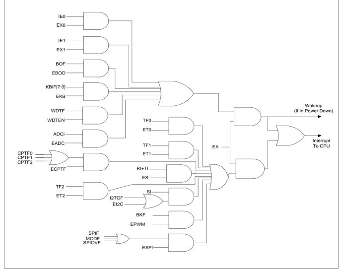
Figure 19-1 Interrupt Flag Block Diagram
