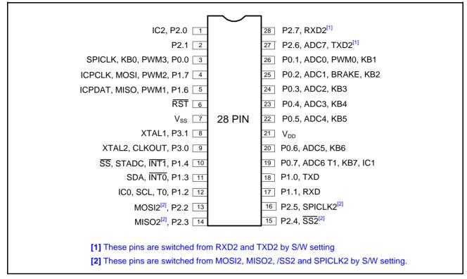
Figure 5-1 TSSOP/SOP 28-pin Assignment
