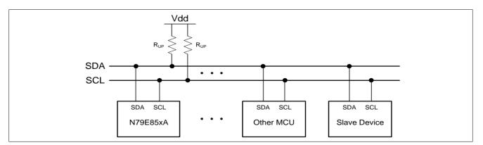
Figure 16–1 I<sup>2</sup>C Bus Interconnection
