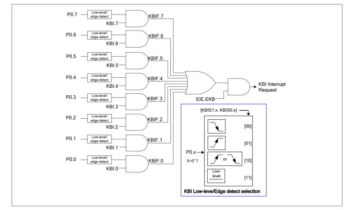
Figure 14-1 Keyboard Interrupt Detection
