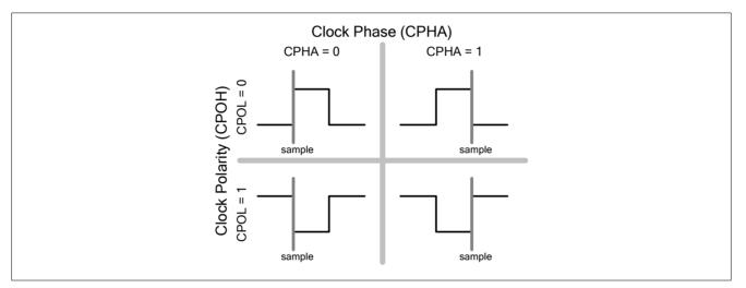
Figure 13-4 SPI Clock Format
