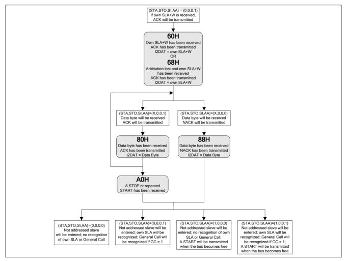
Figure 16–9 Flow and Status of Slave Receiver Mode
