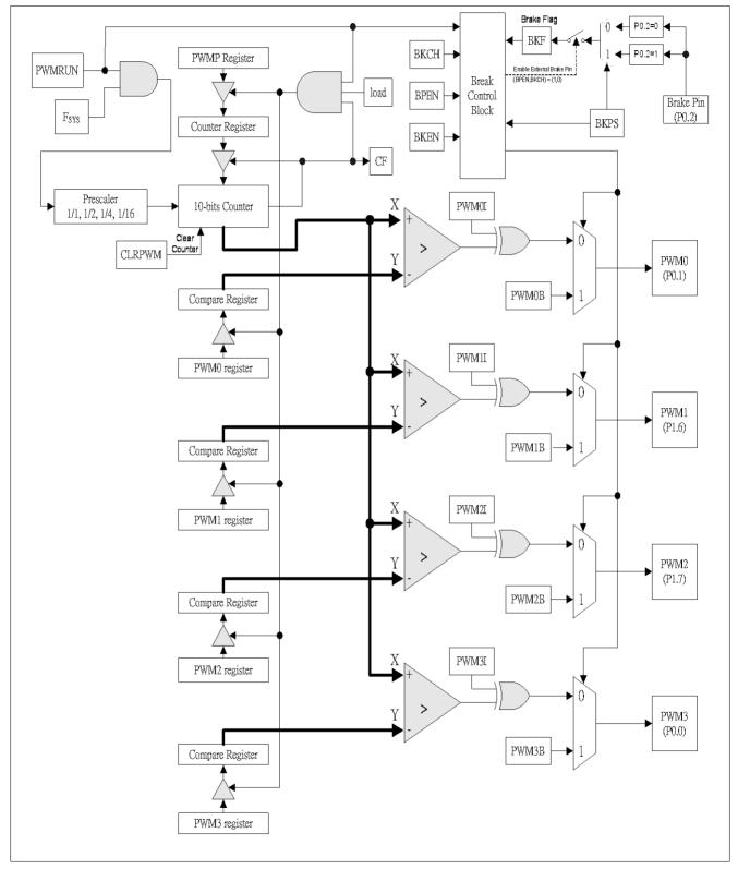
Figure 17-1 PWM Block Diagram
