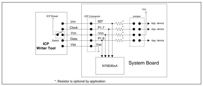
Figure 27–1 ICP Connection with N79E85xA
