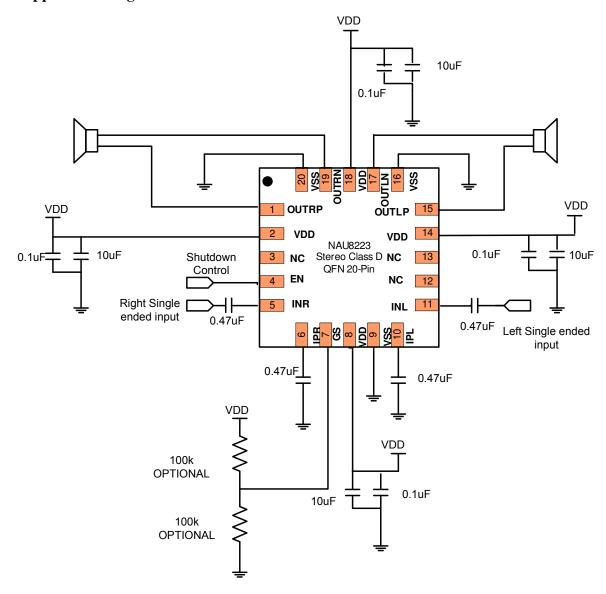
**P.S.** GS Pin – The  $100k\Omega$  resistors are optional. GS can be floating for internal gain setting = 0dB. Please refer Section 2.1 (Gain Setting) for the detailed explanation.
