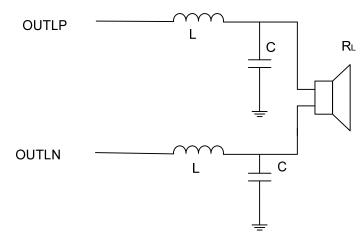
NAU8223 outputs connected to speaker with LC filter
