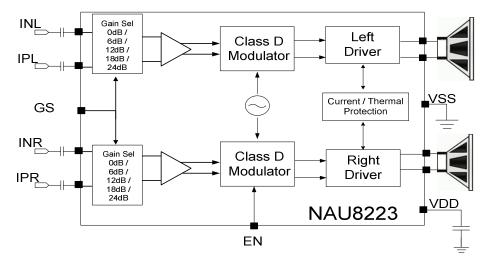
Figure 1: NAU8223Block Diagram
