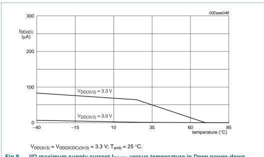
Fig 8. I/O maximum supply current I<sub>DD(IO)</sub> versus temperature in Deep power-down mode
