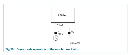
In slave mode the input clock signal should be coupled by means of a capacitor of 100 pF (Figure 29), with an amplitude between 200 mV (RMS) and 1000 mV (RMS). This corresponds to a square wave signal with a signal swing of between 280 mV and 1.4 V. The XTAL2 pin in this configuration can be left unconnected.
