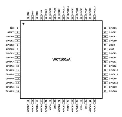
Figure 4. WCT1001/3AVLH Pinout Diagram
