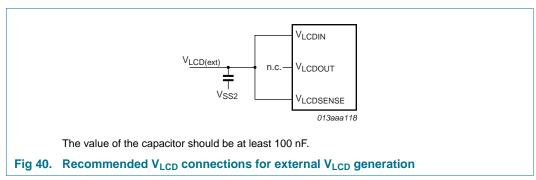
**Remark:** When using an external  $V_{LCD}$ , the internal  $V_{LCD}$  generator **must never** be switched on and direct mode must be avoided otherwise damages will occur.
