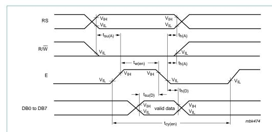
Fig 34. Parallel bus write operation sequence; writing data from microcontroller to PCF2119x
