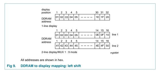
When data is written to or read from the DDRAM, wrap-around occurs from the end of one line to the start of the next line. When the display is shifted each line wraps around within itself, independently of the others. Thus all lines are shifted and wrapped around together. The address ranges and wrap-around operations for the various modes are shown in Table 8.
