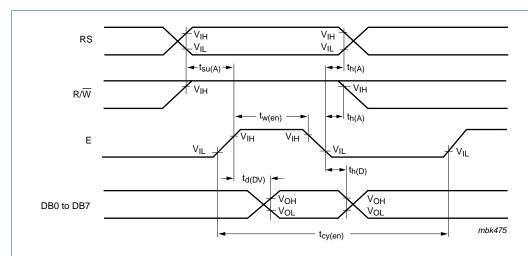
Fig 35. Parallel bus read operation sequence; writing data from PCF2119x to microcontroller
