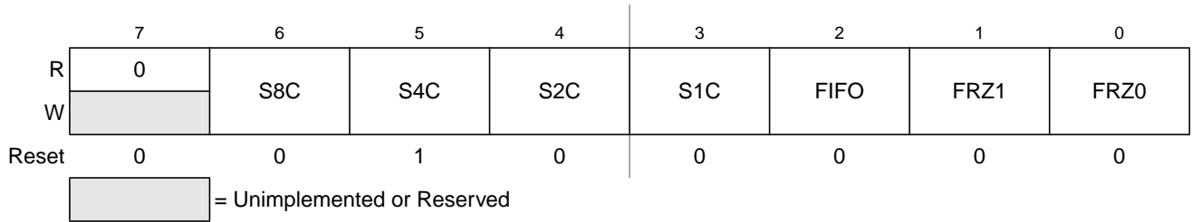
Figure 4-6. ATD Control Register 3 (ATDCTL3)
