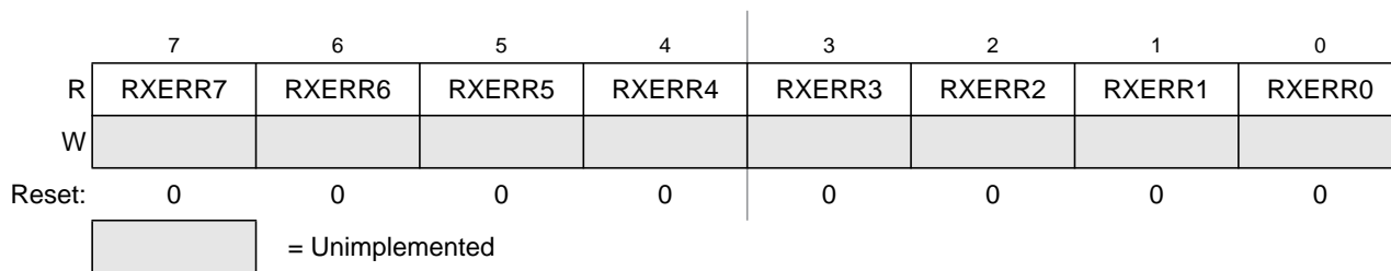
Figure 10-18. MSCAN Receive Error Counter (CANRXERR)
