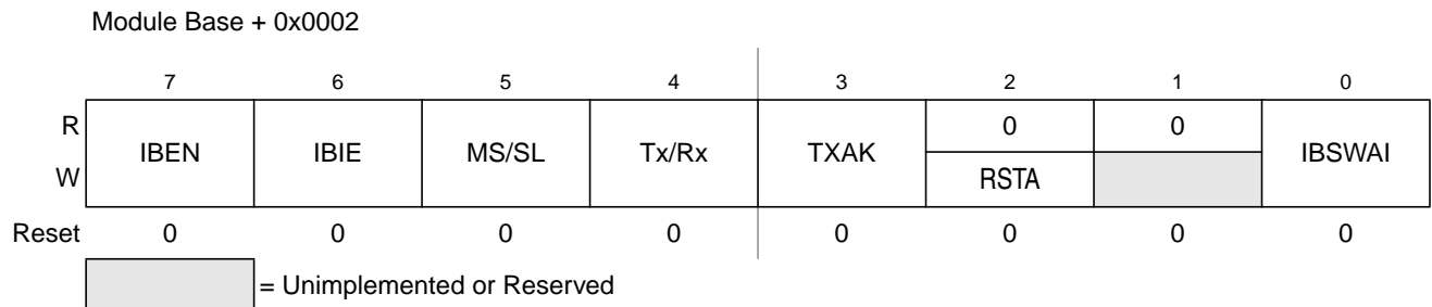
Figure 12-6. IIC Bus Control Register (IBCR)
