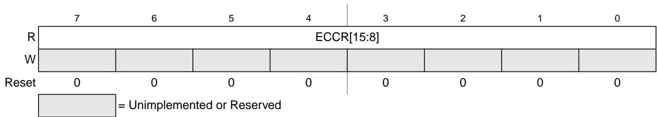
Figure 19-20. Flash ECC Error Results High Register (FECCRHI)
