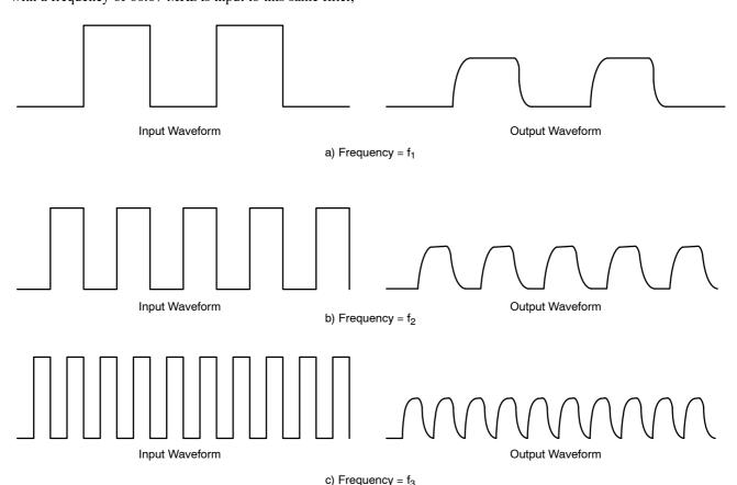
Figure 5. Input and Output Waveforms of Filter
